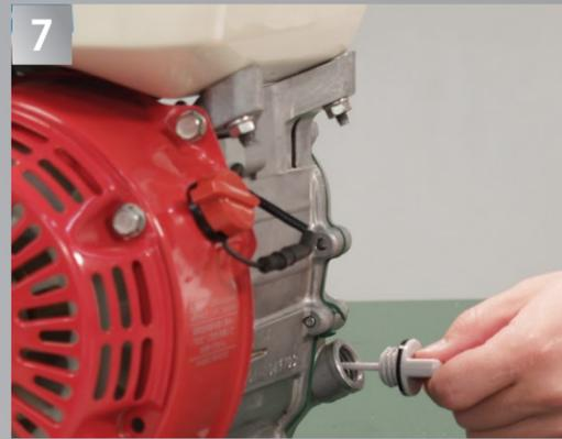
Reinstall the oil filler cap/dipstick.
