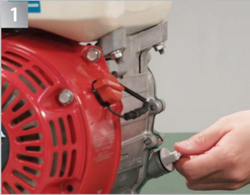
With the engine on a level surface, remove the oil filler cap/dipstick.
