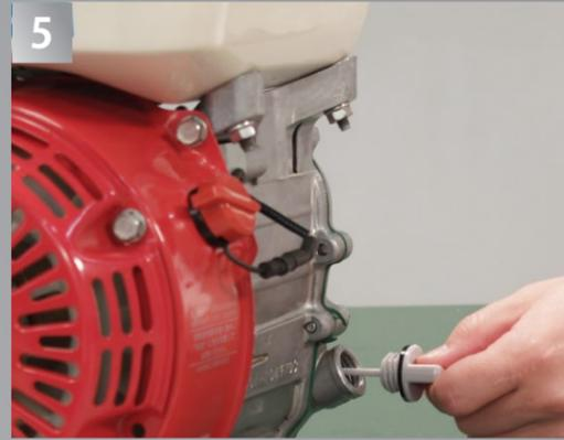
Insert the oil filler cap/dipstick into the oil filler neck as shown, but do not screw it in.
