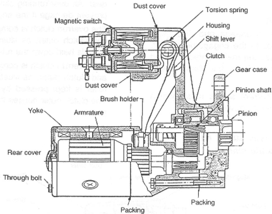
1) Construction of the reduction type starter motor
