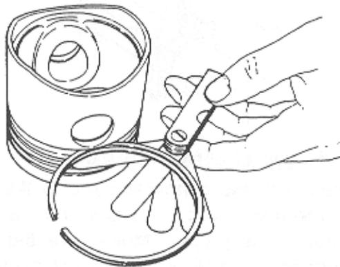
**Measuring the clearance between the piston ring and groove (Side clearance)**
