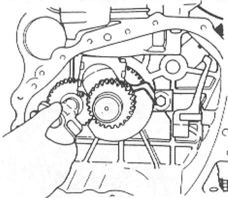
Removing the balancer shaft
