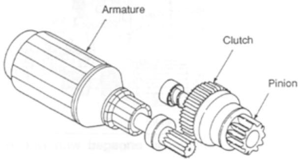
To prevent the motor from being affected by a shock when the engine starts and over-runs, the starter motor has an over-running clutch.
