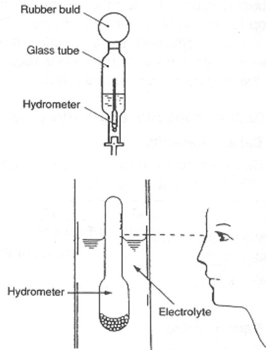
Check the electrolyte level every 7 to 10 days. The electrolyte must be kept 10 – 20 mm (0.3937 – 0.7874 in.) over the top of the plates.
