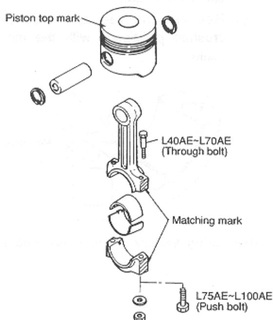
(Line up the piston and connecting rod)
