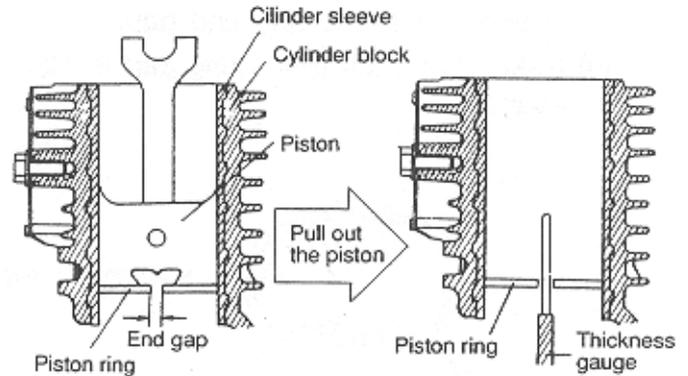
(Push in the piston ring using the piston head)
