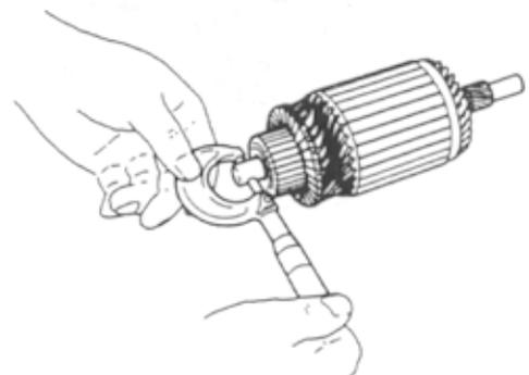
(2) Depth of commutator insulating material
