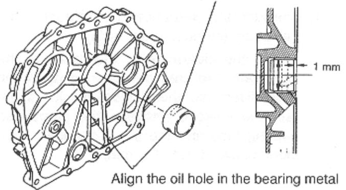
Align the oil hole in the bearing metal with the oil groove.
