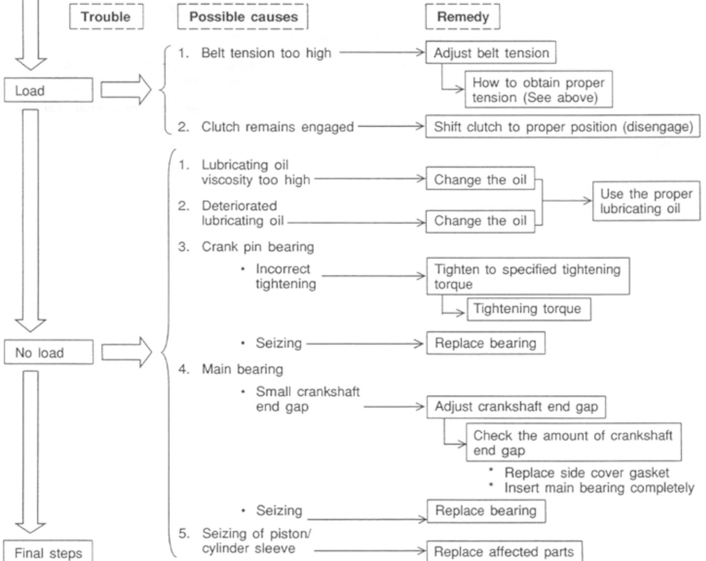
4. **Failure of starter motor (starter)**
