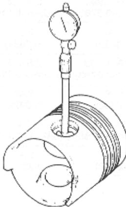
(Checking piston pin hole)
